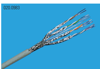
Installation Cable Real10 Cat.6 A , S/FTP, 4P, 650 MHz, LSFRZH, 500 m
