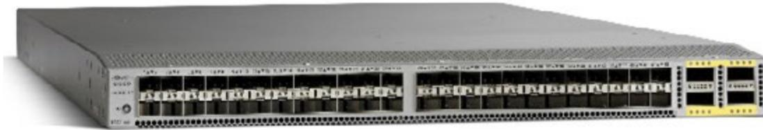
Cisco Nexus 6001 Series 48-Port 10 Gigabit Ethernet SFP+ ports
