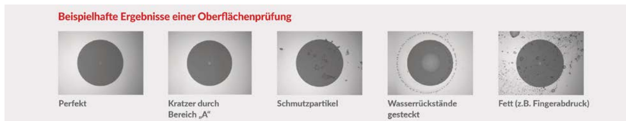
Image 050.6383: How optical fiber contact surfaces look in different states. From left to right: cleaned connection, water residue, dust and dirt particles, fingerprint. Swiss fiber optic specialist R&M recommends that, before pairing, you should always first check fiber optic connections and then clean if necessary. Image source: R&M
